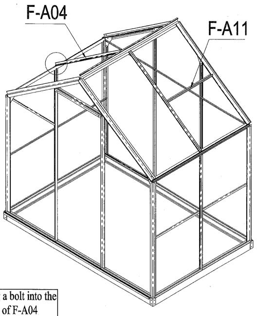
Sliding a bolt into the groove of F-A04
