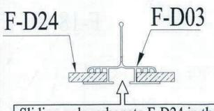
Sliding polycarbonate F-D24 in the channel of profile F-D03.
